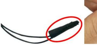
The metal hats on the end of the antenna string are sealed by acetate tape to avoid possible damage to the system.
