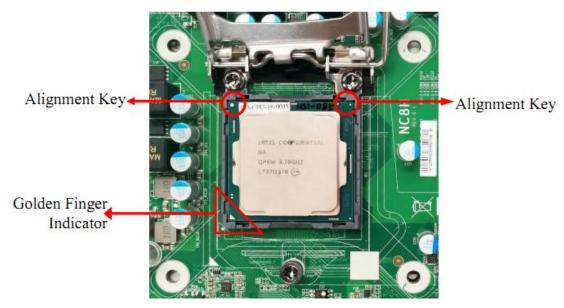
Make sure that Pin-1 Golden Finger Indicator in the place as shown in the above photo and match the two alignment keys on the CPU with two points of the socket. CPU can only be correctly installed in this direction. Incorrect installation might cause damage to CPU.
