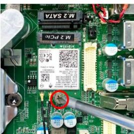
10. If you do not need to install M.2 SATA card, lock the previously removed screw to its original place.
