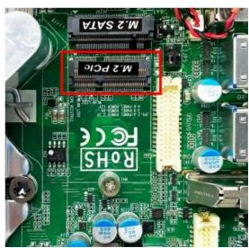
1. Locate the M.2. PCIe, type-2230 slot on the board.
