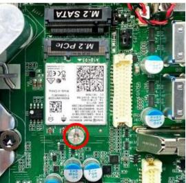
Lock the card to the board by tightening up the screw post to the marked spot.
