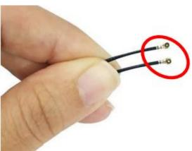
8. Tear off the tape to find metal hats of Wi-Fi antenna string.
