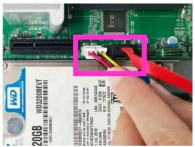
8. Plug the other side cable into the SATA power connector and SATA port connector on the board.
