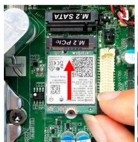
Insert the gold-figure side of compatible card into M.2. PCIe slot. See to it that the goldenfigure side is fully inserted into the slot.
