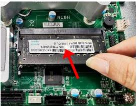
Insert the gold-figure side of the compatible SO-DIMM into the slot at a 30 degree and press down. The eject tabs will lock automatically if installed correctly.
