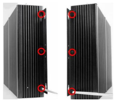
1. Install wall mount rack to the system by tightening the screws in the marked position. Then lock the other three screws on the other side in the same way.
