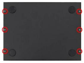
Locate the screws in the spots marked on the top cover of the system and unscrew them one by one.
