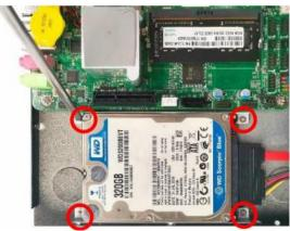
Lock the racks hard disk with SATA HDD installed to its original places by tightening the screws in the marked spots.
