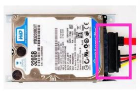
Plug this side of the cable to SATA power-in connector and SATA connector of the hard disk.
