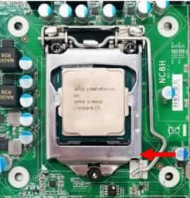
7. Press down the load level and move it leftwards to make sure it is locked under the notch.
