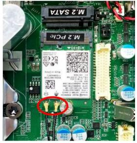
Press the metal hats of the antenna string ends to the antenna slots on the card as showed.
