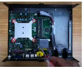
For CPU installation, user needs to remove the screws on the marked spots to dissemble CPU heatsink at the mark position at first.
