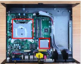
3. When installation finished, tear off the protective film from the greases before assembling the back cover to the chassis.
