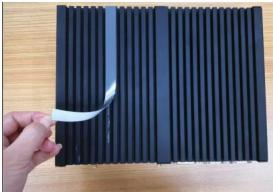
Turn over the chassis with the heatsink side upwards. Remove the silver Myra sticker on the heatsink.
